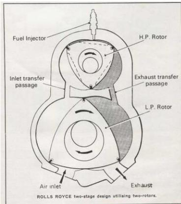
FM initially designed, built, and dyno tested a 294cc compound rotary engine using a 530cc compression/expansion (CE) rotor in a design similar to Rolls-Royce.
