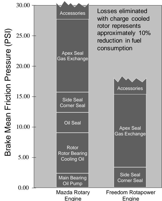
Figure 1: Comparison of Friction Losses between the Mazda 500cc rotary engine and the Freedom 530cc Rotapower engine<sup>5</sup>
